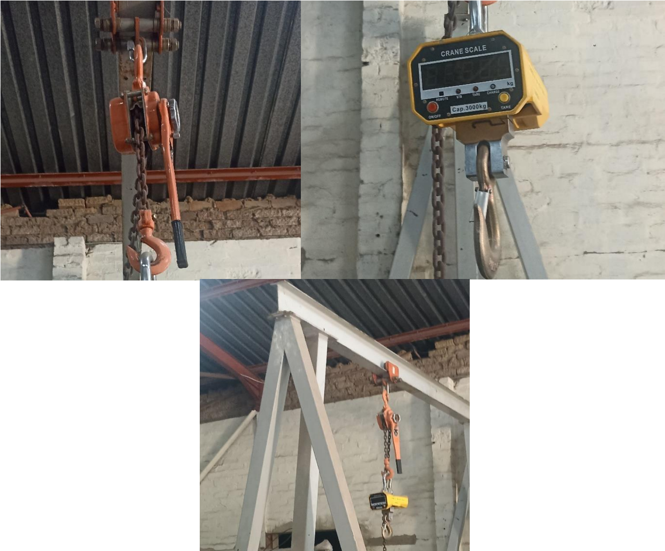
Figure 34: Drop Test Crane, Weight Scale and Lever Block Set Up
