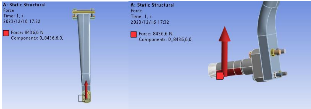
Figure 31: Taildragger Aircraft Level Landing Load Application (Deflection Validation)
