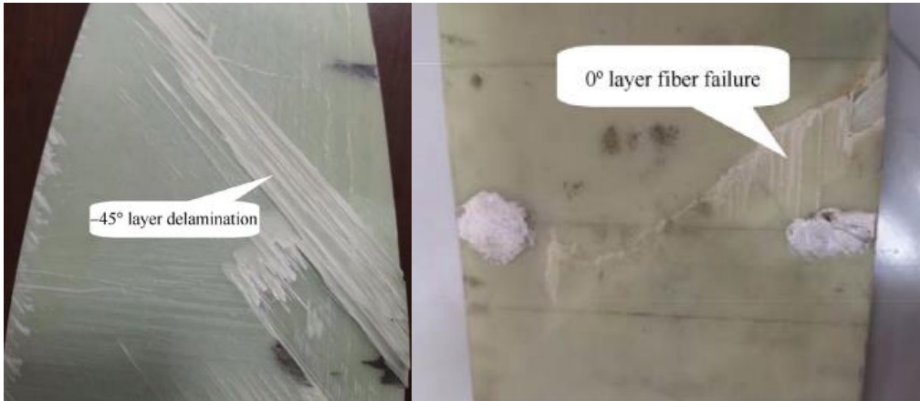
Figure 22: Tensile Failure on Landing Gear [11]
