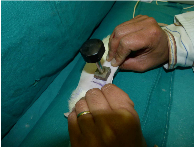
Figure 1 : Placement of the 2 x 2 cm brass block placed for a period of 10 secs on skin that was tented out to get an even contact.
