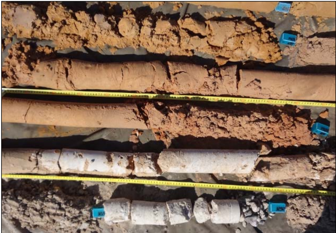
Figure 28: The range of Kalahari sand colours, orange in the top row and darker red-orange in the second and third row. A calcrete lens is visible in the fourth row and gravels in the bottom row on the right-hand side of the photo.
