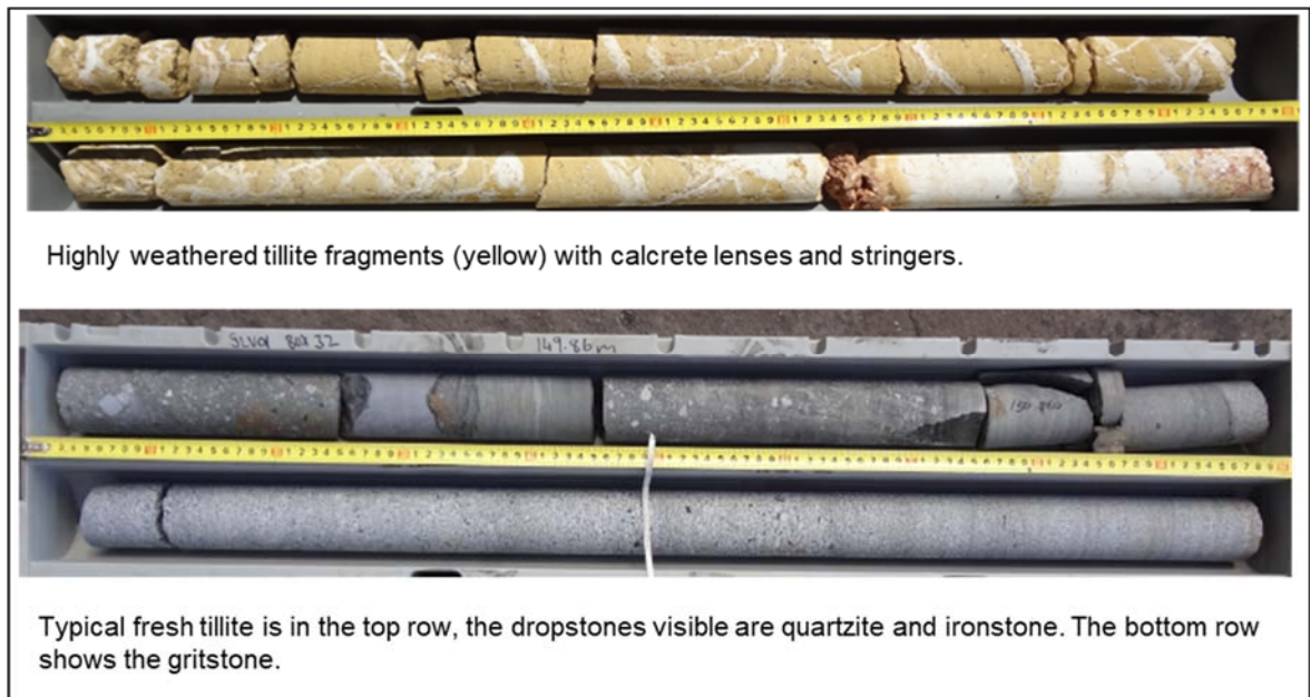
Figure 30: Highly weathered and fresh tillite
