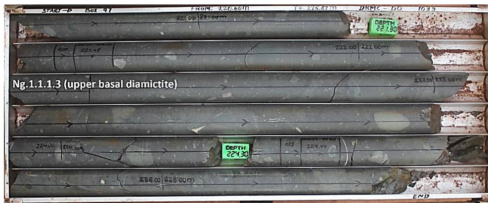
Figure 31: Upper basal diamictite from DKMC_DD1039 at 221.00 m.
