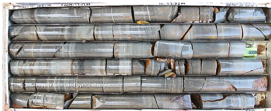
Figure 34: Upper laminated pyritic siltstone and sandstone from DKMC_DD624 at 80.00 m.
