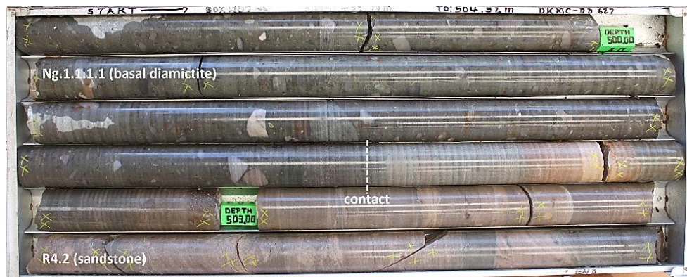
Figure 29: Contact of R4.2 sandstone and lower basal diamictite from DKMC_DD627 at 500.00 m.
