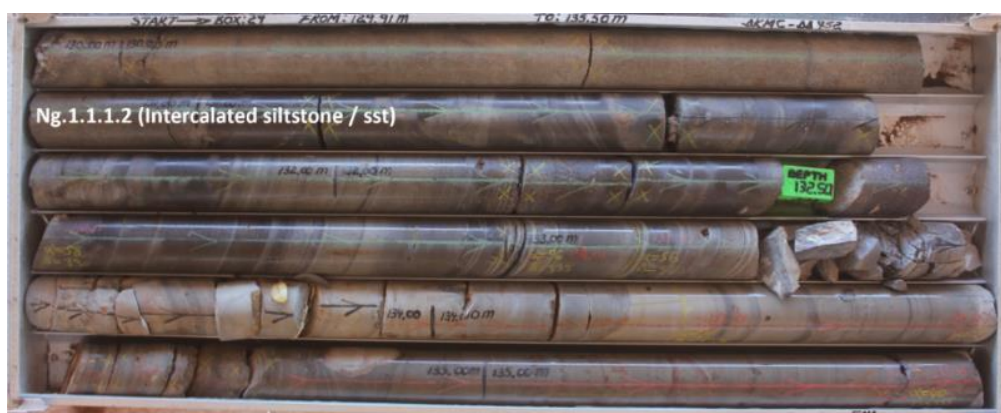
Figure 30: Intercalated siltstone and sandstone from DKMC_DD952 at 132.50 m.
