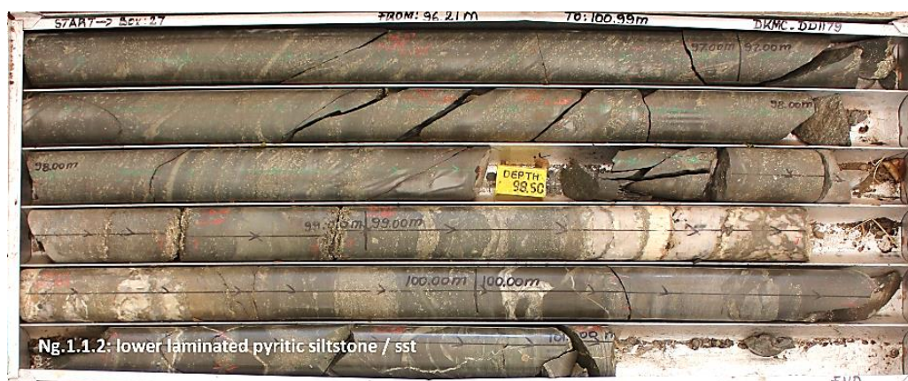
Figure 32: Laminated pyritic siltstone from DKMC_DD1179 at 98.00 m.
