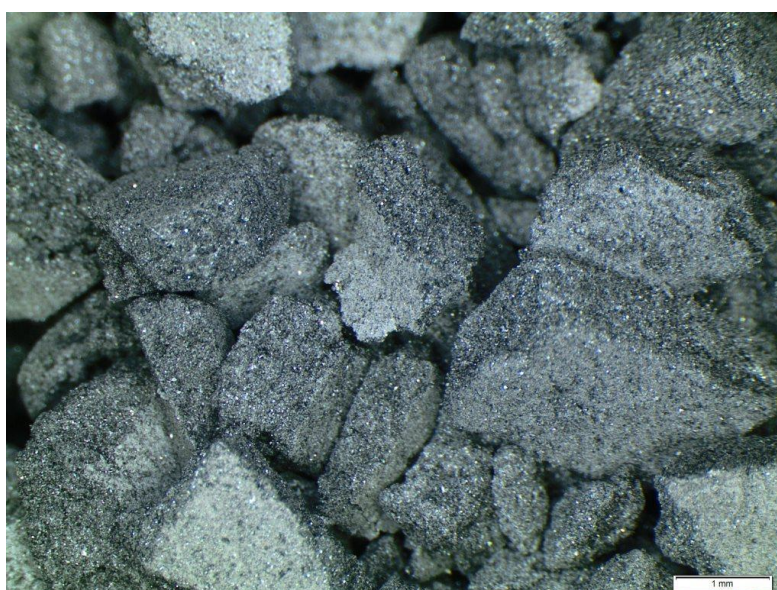
Figure 54 GMS granule particles used for uniaxial pressing GMS slugs.
