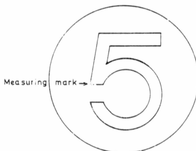
FIGURE A.2 Sketch illustrating how the control points on the reference grid were co-ordinated in the Wild A7 Autograph.
