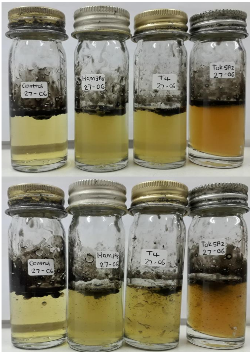
Figure 3.2: MacConkey 24 hour degradation assay results for three strains analysed in Chapter 3. Left to right: negative control, G. thermodenitrificans Ham3A8 and DSM 465 T , and G. stearothermophilus Tok5A2, before agitation (top) and after agitation (bottom).
