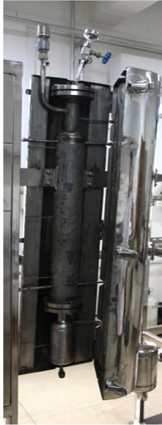
Figure 8-3 Diagram of the bench scale reactor used in the BTL facility
