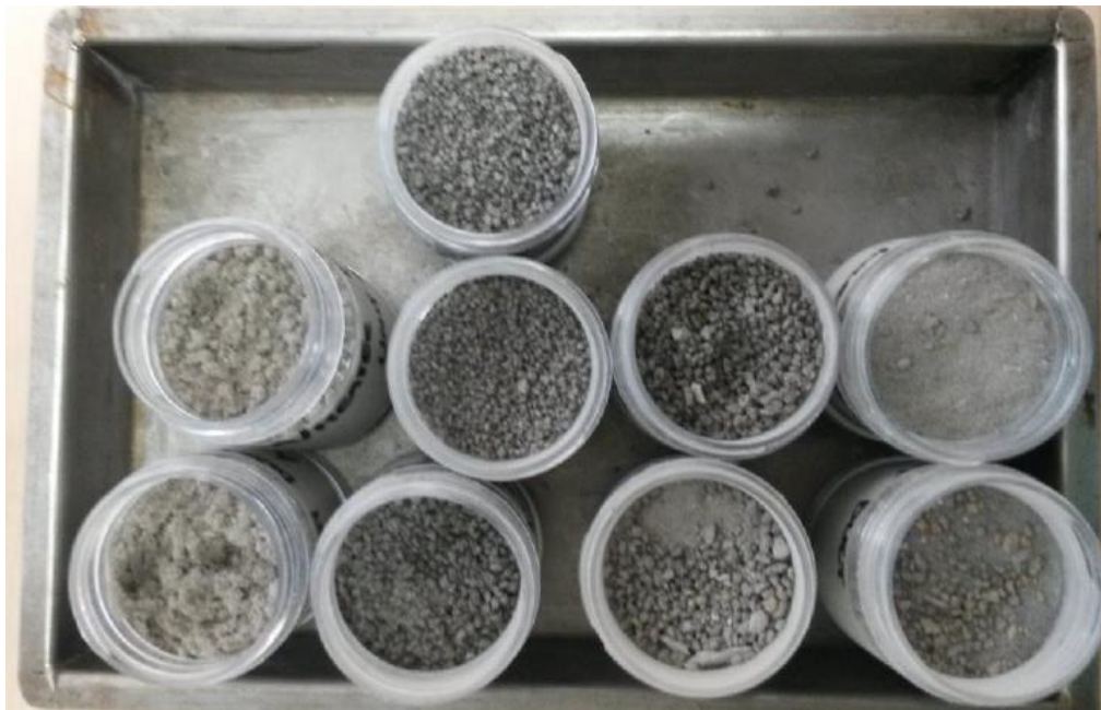
Figure 1.4: Visual features of the different air heater ash deposits. (Van Alphen, 2018)
