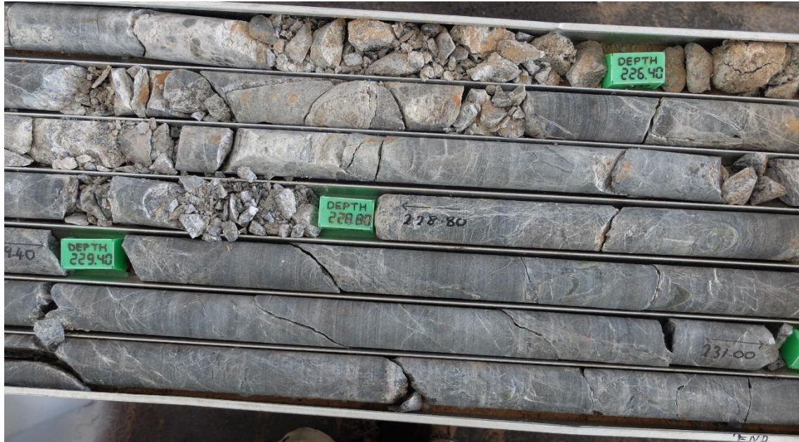
Figure 5: Altered ultramafic rocks in borehole KKME 1-6, from \sim 226 m to \sim 232 m depth. Core diameter is 4.76 cm (NQ)
