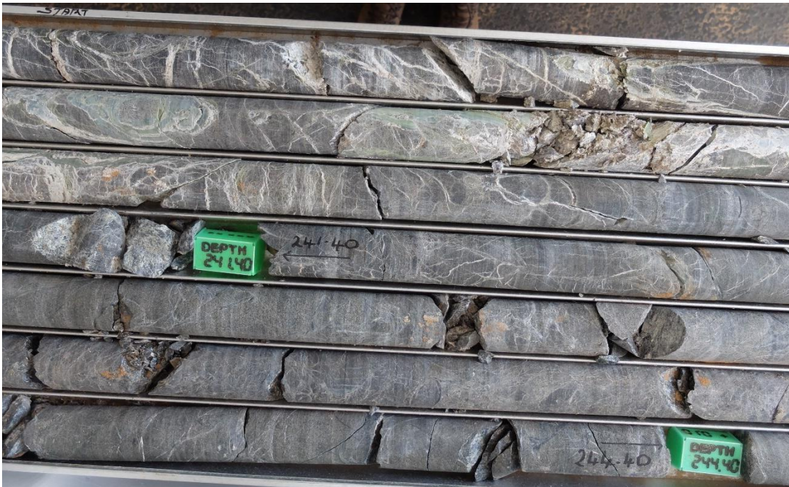
Figure 6: Serpentine and talc veining in ultramafic rocks in borehole KKME 1-6, from ~239m to ~244.5m depth. Core diameter is 4.76 cm (NQ).
