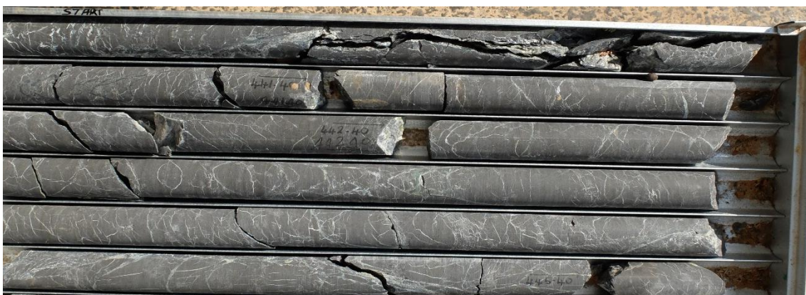
Figure 8: Talc and serpentine veinings in serpentinite in borehole KKME 1-6, from ~440m to ~446.5m depth where samples IMK – 05156 used in microprobe and the TIMA is located. Core diameter is NQ.
