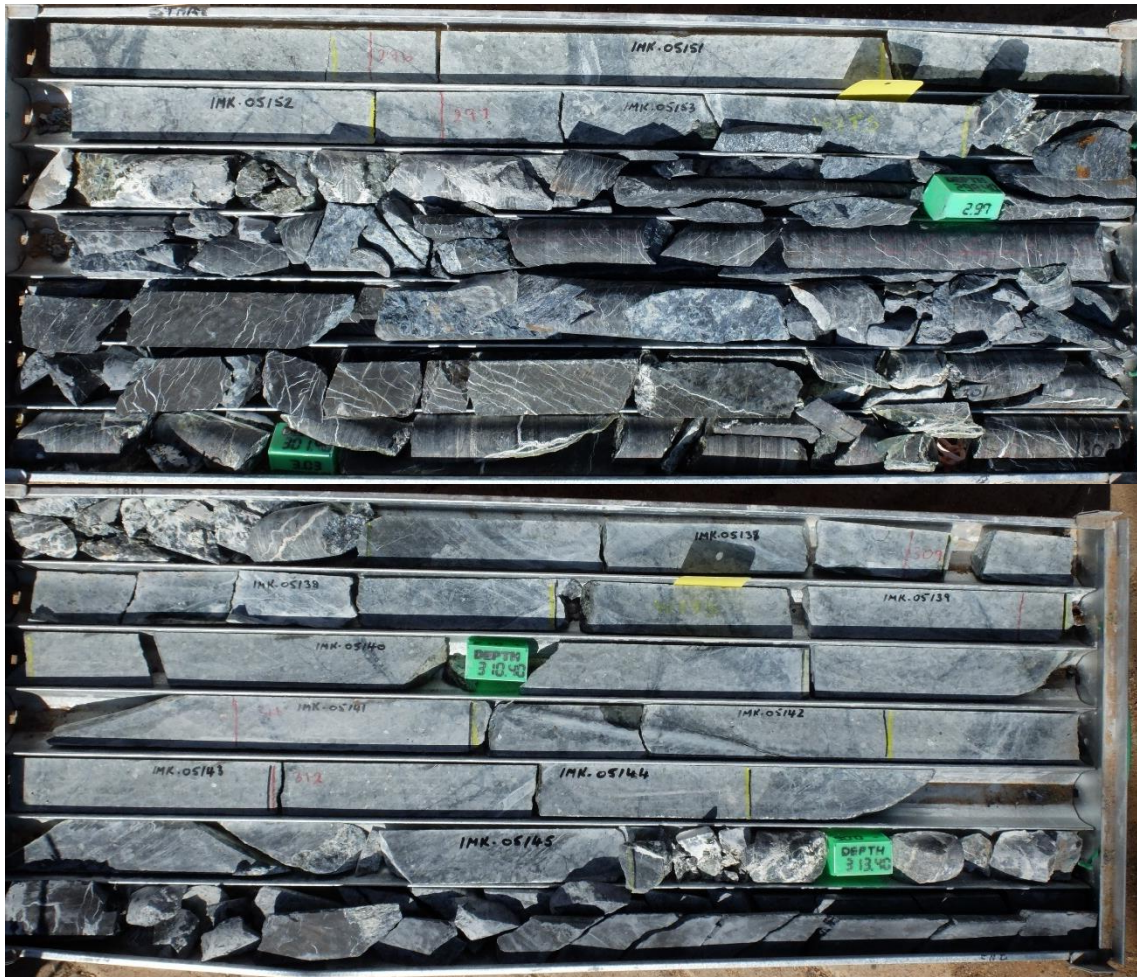
Figure 7: Fractured core in a fault zone in borehole KKME 1-6, from ~296m to ~302m and ~308 to ~315 m depth where mineralised samples IMK – 05139 and IMK – 05149 used in microprobe and the TIMA are located. Core diameter is NQ.
