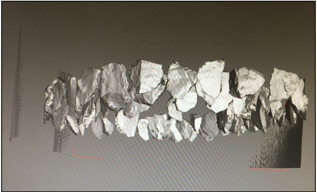
Figure 3.7. Tray 1 showing walls of plastic tubing picked up during a scan.
