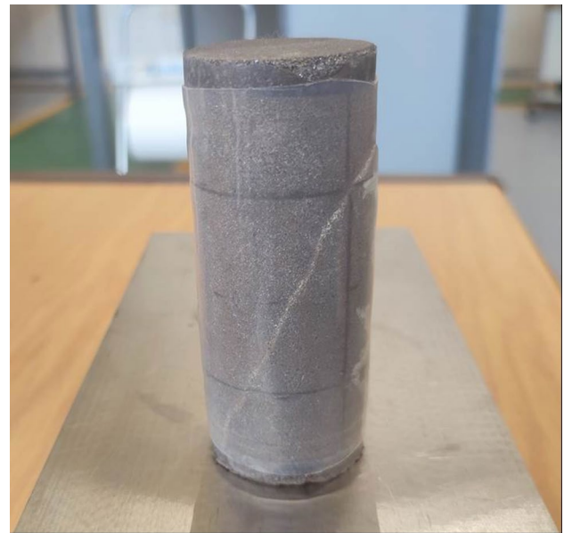
Fig. 9 Shear failure observed in triaxial tests
