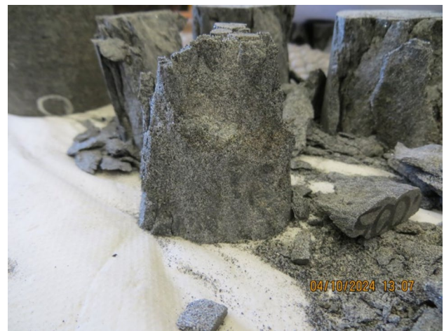
Fig. 10 Shear failure observed in uniaxial tests (w/h ratio=0.4)
