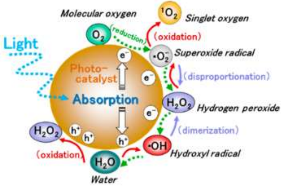
Figure 2.5. ROS generated during TiO_2 photocatalysis [55].
