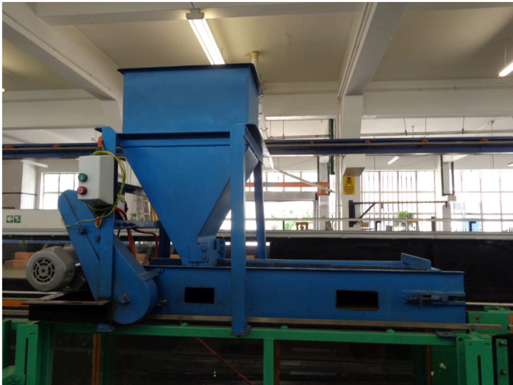
Figure 3-3 Side view of sediment feeder mounted on flume
