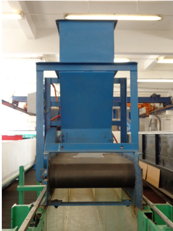
Figure 3-4 Front view of sediment feeder mounted on flume
