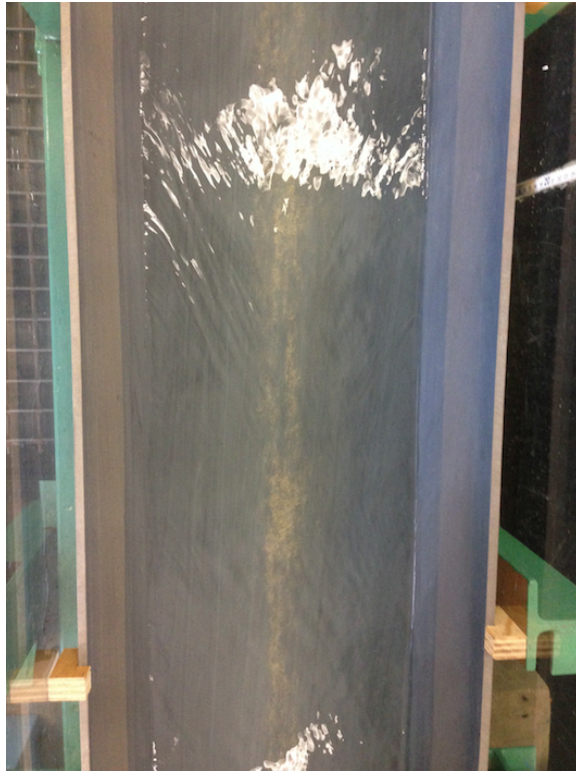
Figure 3-12 Discrete bed load movement
