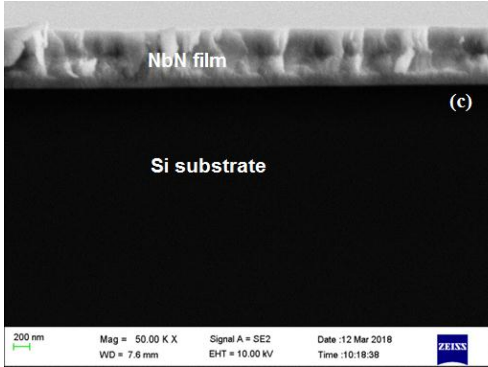
Figure 5.3: SEM micrographs of surface morphology of NbN films deposited at sputter power of 200 W for (a) 9 mins, (b) 19 mins, and (c) 33 mins. Film (a) corresponds to Zone I, while (b) and (c) correspond to Zone III of the structure zone model.
