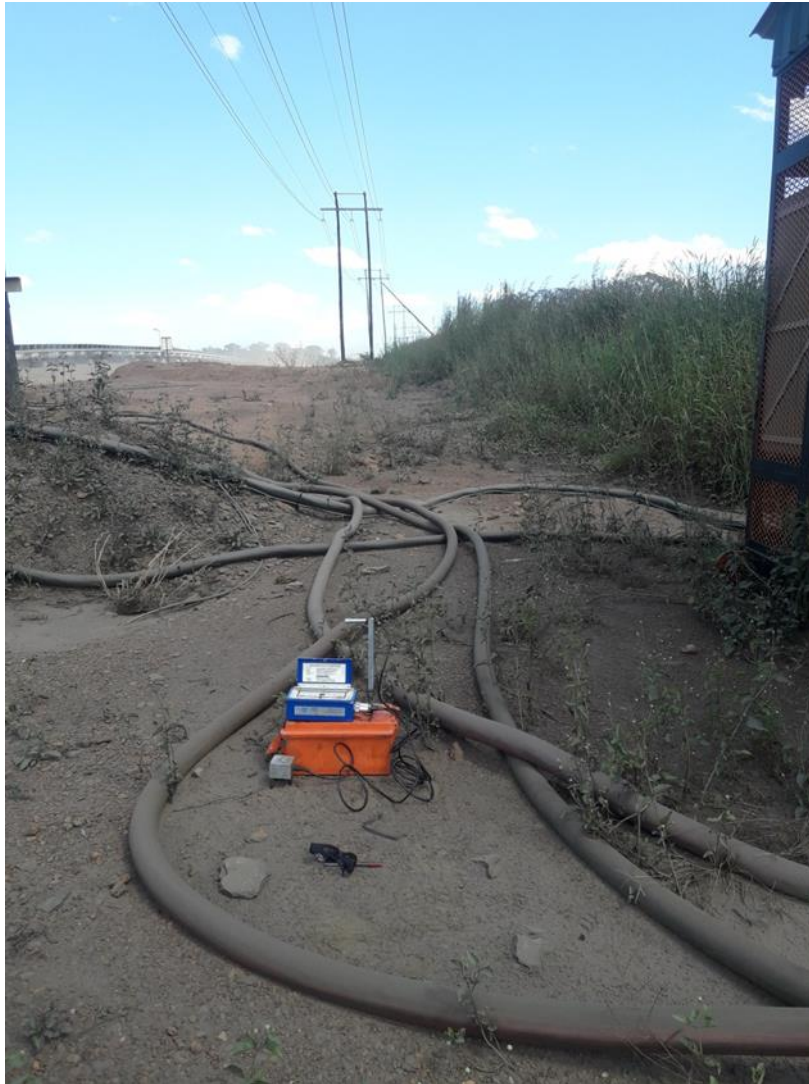
Figure F-1: Set up of the seismograph at the power substation above the western wall
