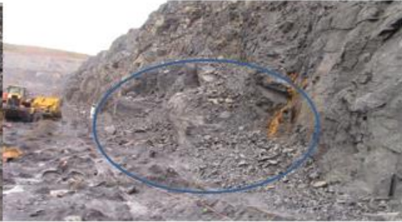
Toe burden not blasted caused by poor charging or poor drilling
