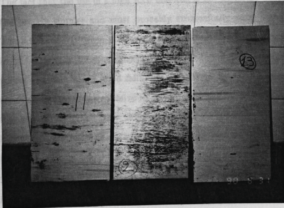
Photograph 5 The reduction of bleeding by using hardwood surface veneers.
