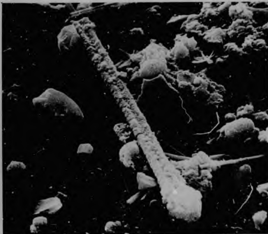
FIG 6.3 Residue from lung of asbestos miner. (Photograph taken on Cambridge Stereoscan Electron Microscopy Dept. University of Witwatersrand. (x4000)
