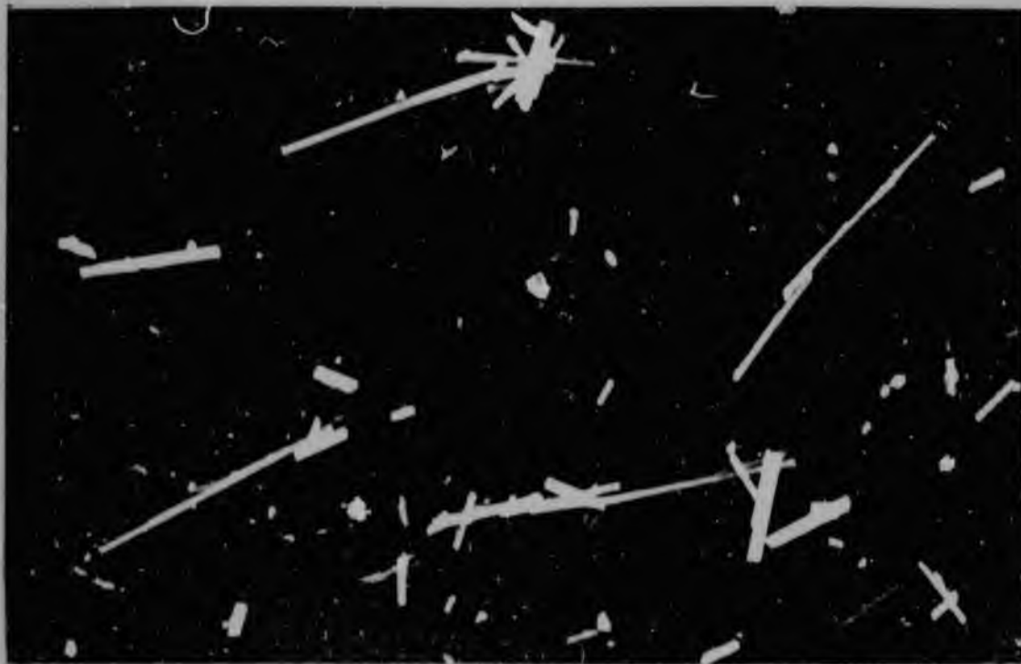
FIG 7.3.5.1 SEM photograph used to determine limit of resolution of light microscope. Fibres circled were invisible under LM.
