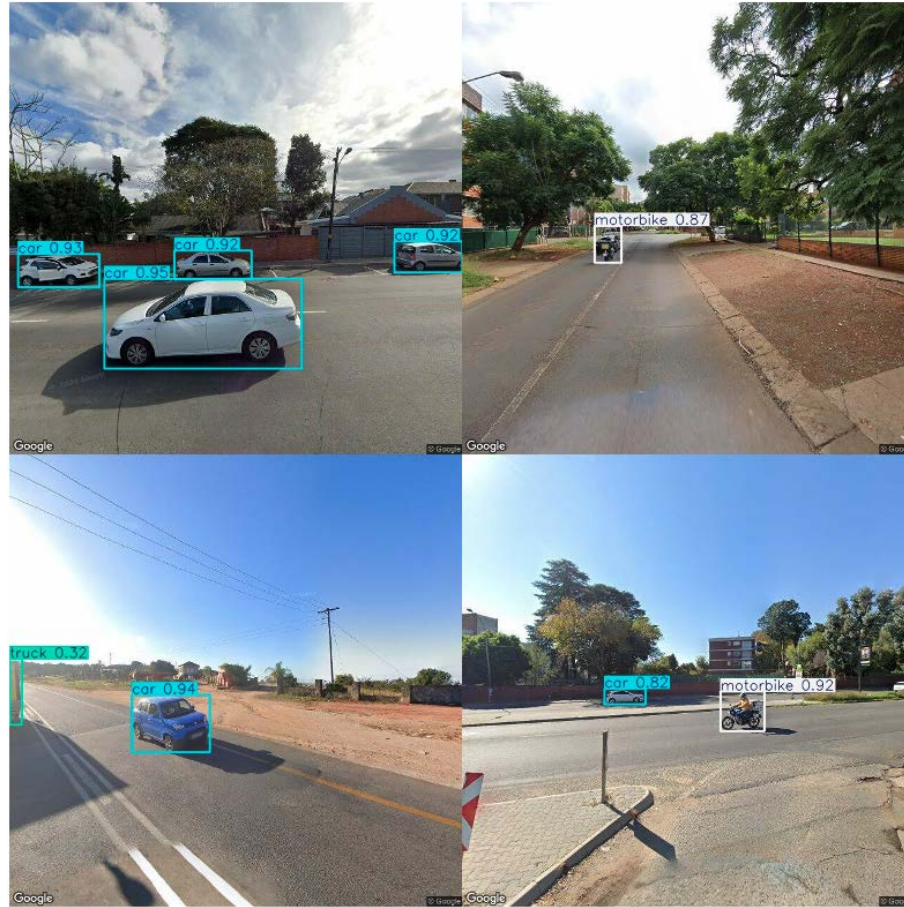
FIGURE 4.7: Images showing high vehicle detection confidence regardless of image variation
