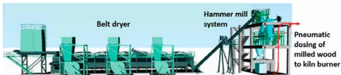
8 Wood biomass processing for lime kiln firing [19]
