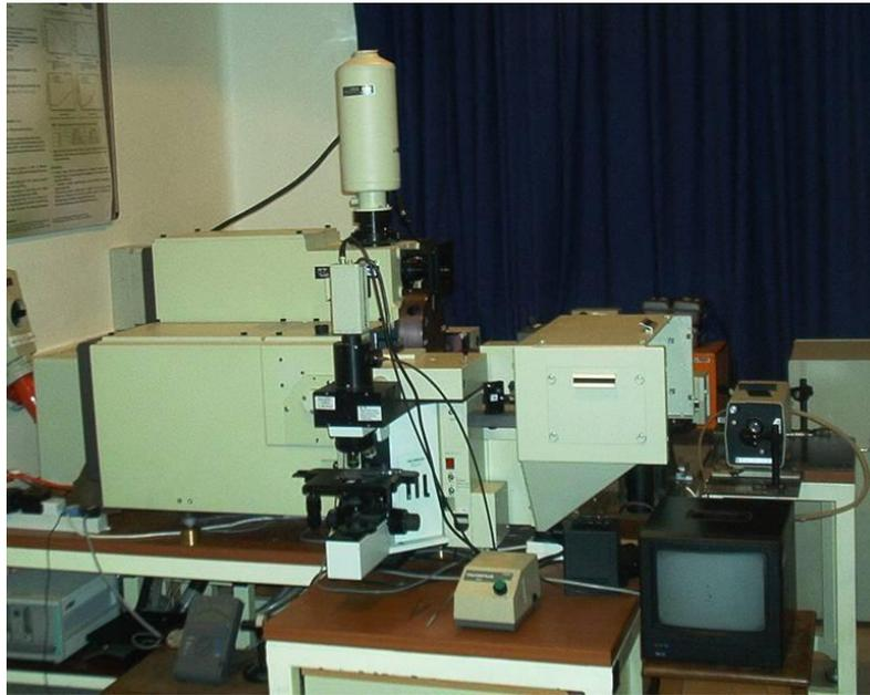
**Figure 4.21** Raman spectroscopy/PL setup at the University of the Witwatersrand.
