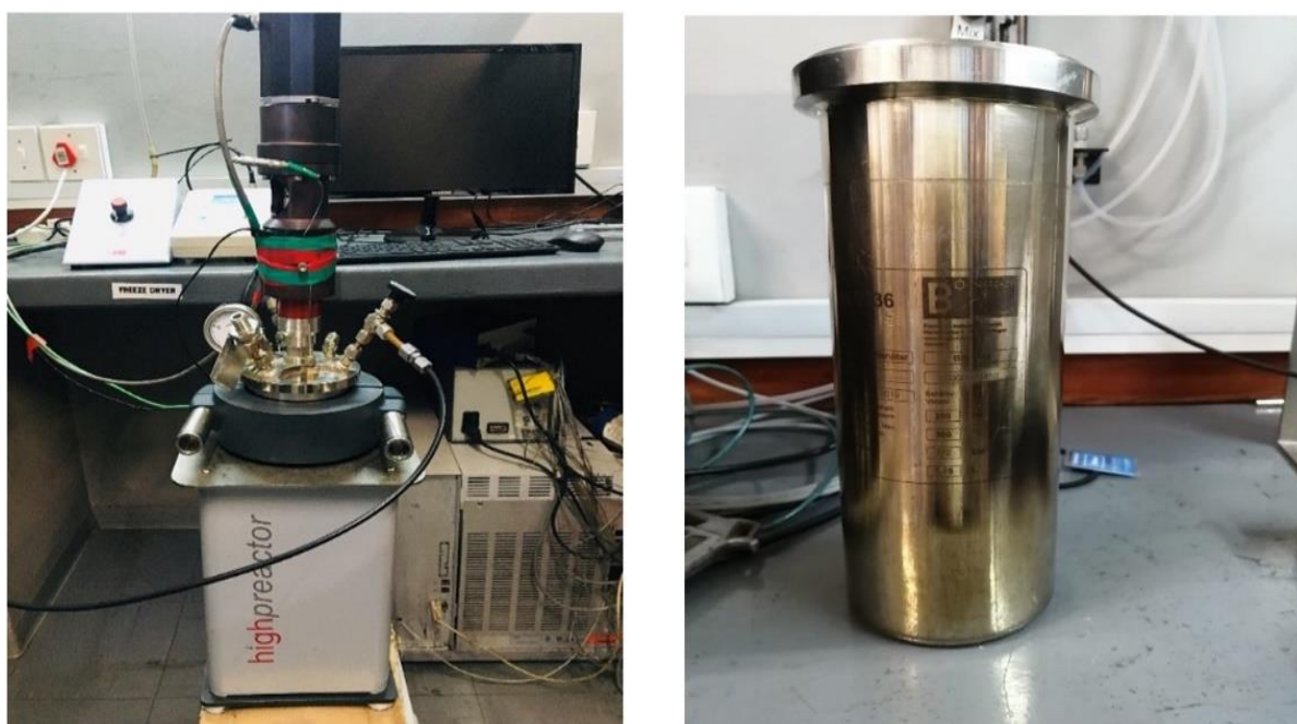
Figure 3.2: Berghof stirring system axis and stainless-steel reactor vessel
