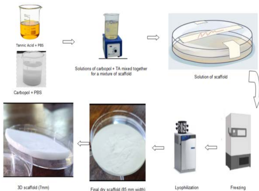
Figure 3-2 Schematic representation of scaffold synthesis of carbopol and tannic acid, and characterization of these polymers.
