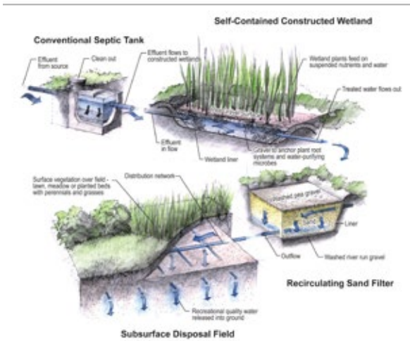
Fig 8.19 "Constructed Wetland Sketch Diagram" 2009
