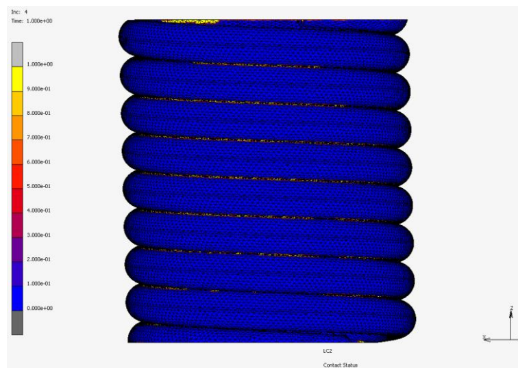
Figure 4.27 Contact status of the inner spring when subjected to the maximum dynamic force.
