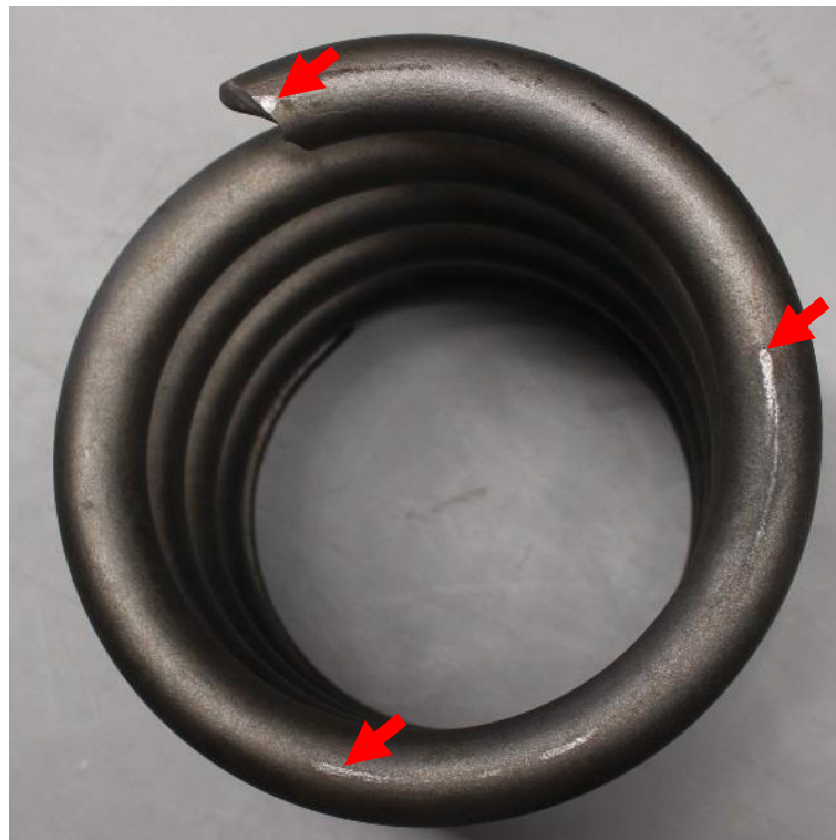
Figure 4.5 Top view of the failed spring.
