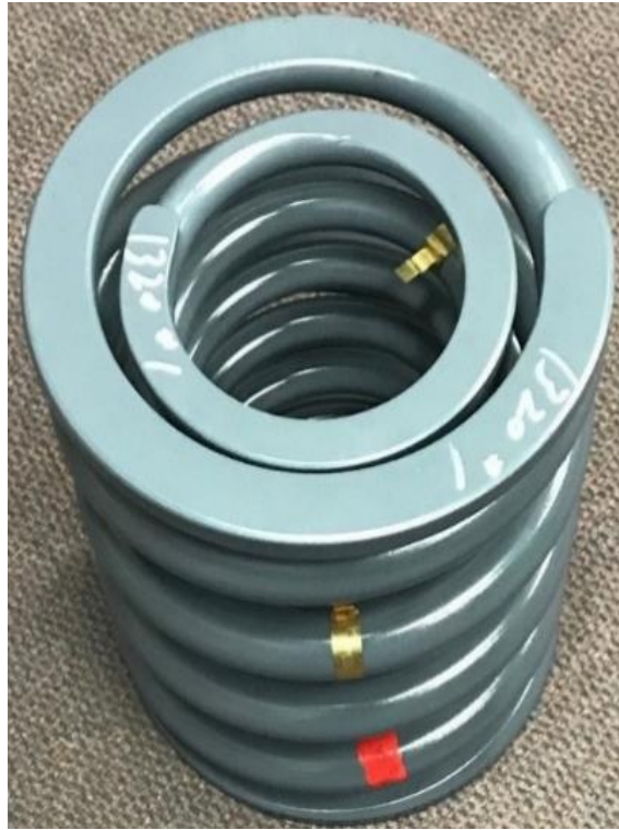
Figure 1.2 A brand new dual helical compression spring used on a 22E locomotive.
