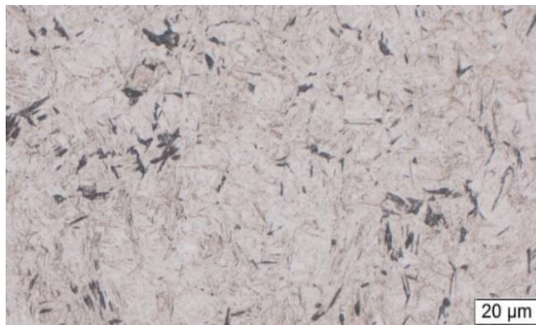
Figure 4.10 Microstructure of the steel after quenching in the Unused oil.
