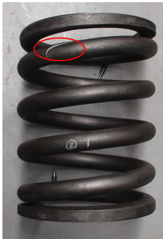
Figure 4.3 Spring that failed during fatigue testing.
