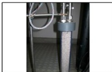
d. Zeolite packed bed to trap degassed volatiles
