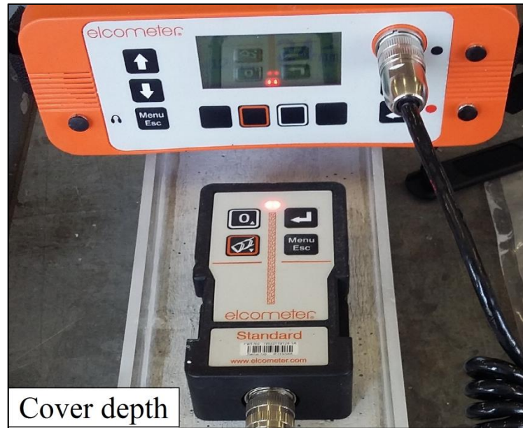
Figure 3.12: Cover depth testing
