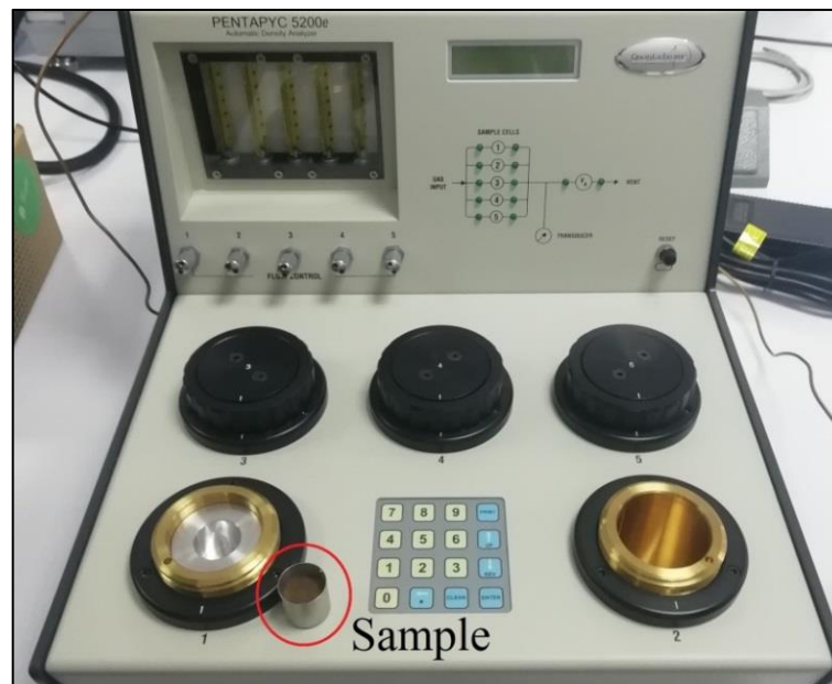
Figure 3.1: Binder density measurement apparatus
