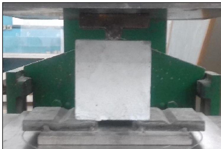
Figure 3.22: Cube fracturing set-up
