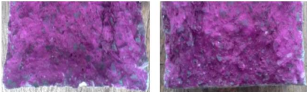
Figure 4.17: Baseline of the carbonation depths
