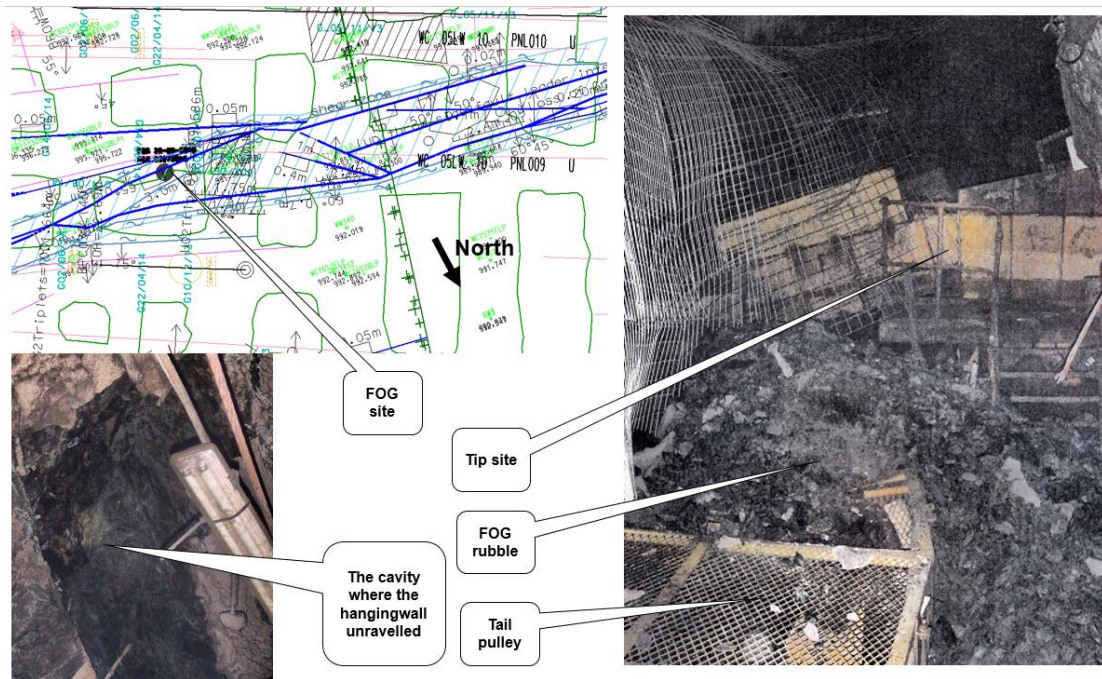
Figure 6-5. FOG that occurred from a vertically inclined shear zone at Central shaft strike 5W bord 5 (Matsobane, 2016d).
