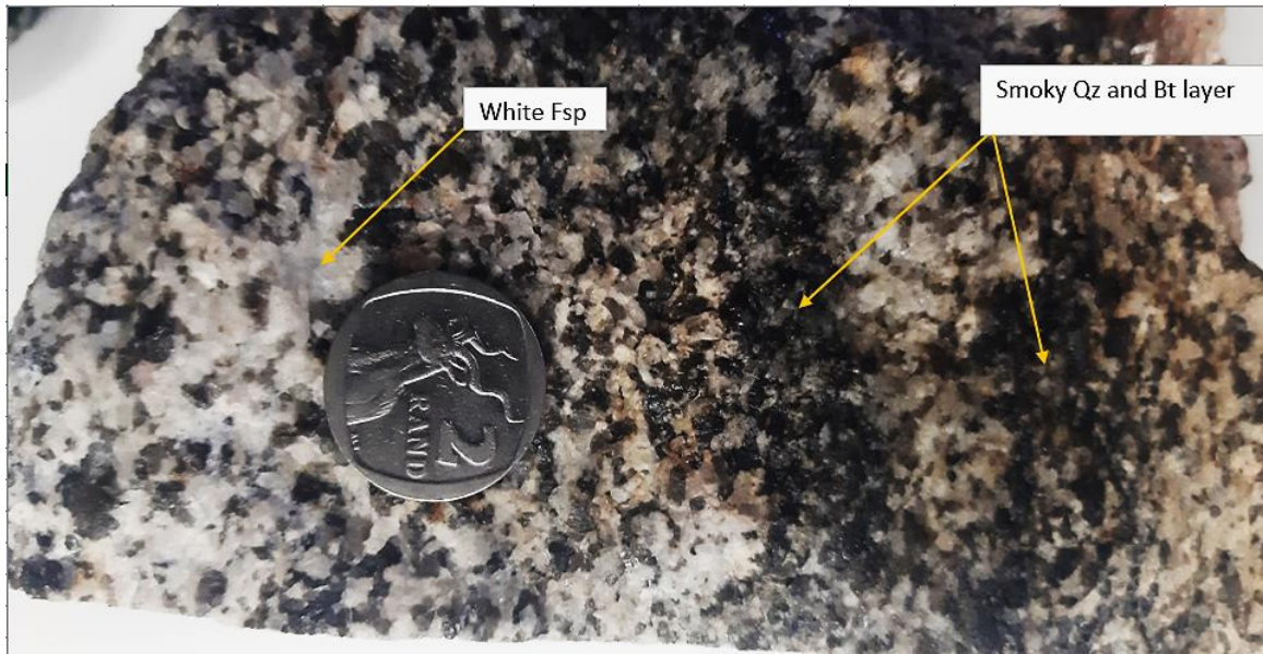
Figure 4.5: TS1 section 4 shows some banding- smoky quartz and biotite forming dark layers.
