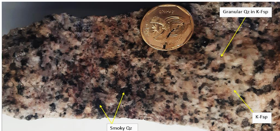
Figure 4.10: E-type section of sample TS2 showing mineral association of smoky quartz and pink feldspar.
