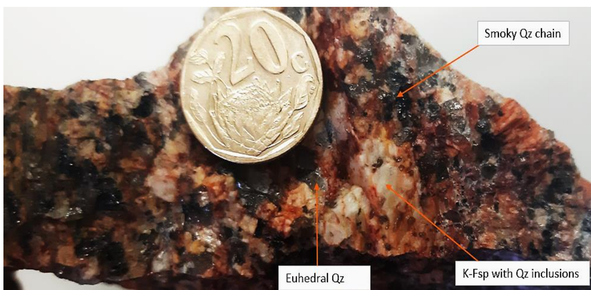
Figure 4.8: Cross-section of oxidation halo section showing the core zone being dominated by pink feldspar while the boundary zone is dominated by smoky quartz.
