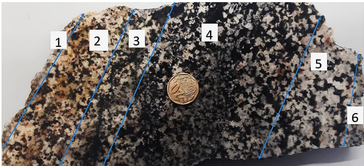
Figure 3.1: Photograph of sample TS1 shows sections division of D-type SLG based on textural variations: TS1 sections 1, 3 and 6 (medium-grained), TS1 sections 2 and 5 (pegmatitic), TS1 section 4 (coarse).
