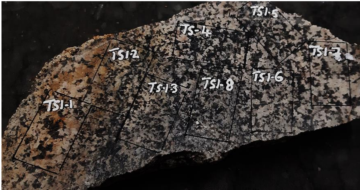
Figure 3.2: Hand specimen of rock sample TS1 (D-type SLG) shows the demarcation for thin section preparation.
