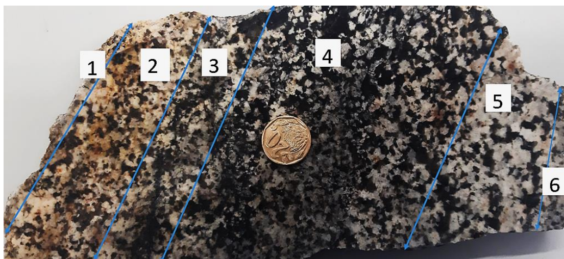
Figure 4.3: Photograph of sample TS1 showing the division of D-type SLG based on textural variations; TS1 sections 1, 3 and 6, TS1 sections 2 and 5, TS1 section 4
