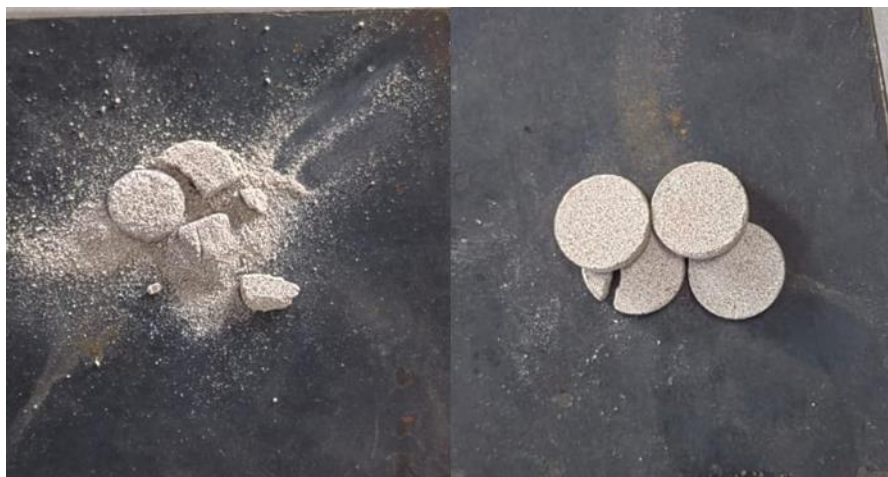
Figure C.7: The combusted composites that were pyrolysed in air
