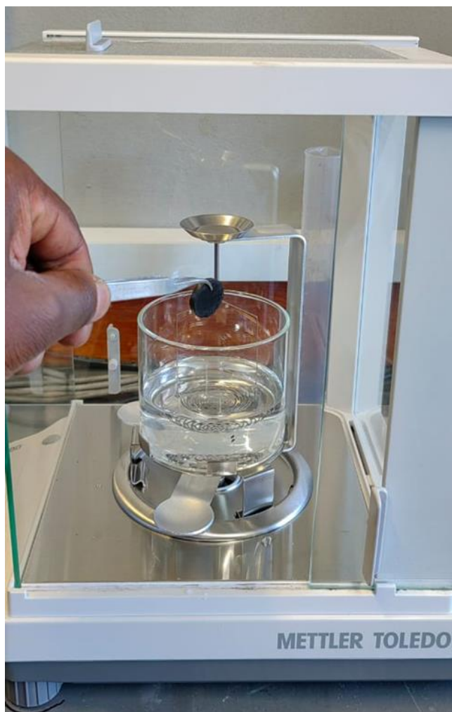
Figure C.10: Weighing suspended mass after water immersion test to determine the mass of the composites in water
