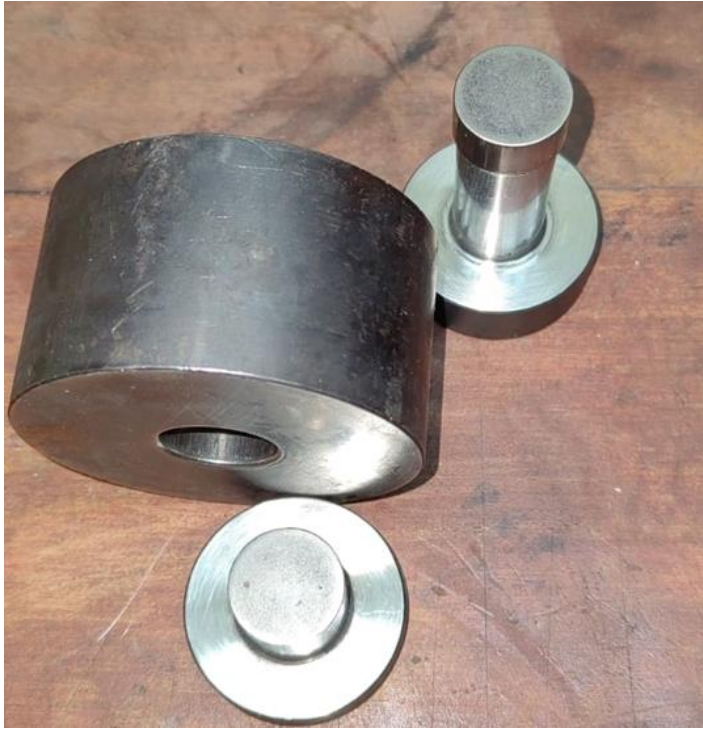
Figure C.3: Cylindrical mould used to produce small composites
