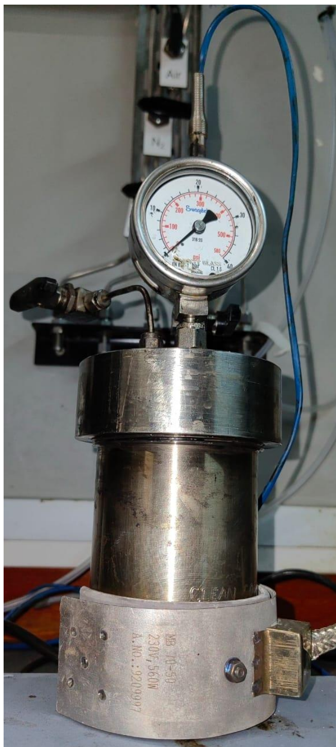
Figure C.2: Stainless steel thermal reactor used to produce coal tar pitch from coal tar
