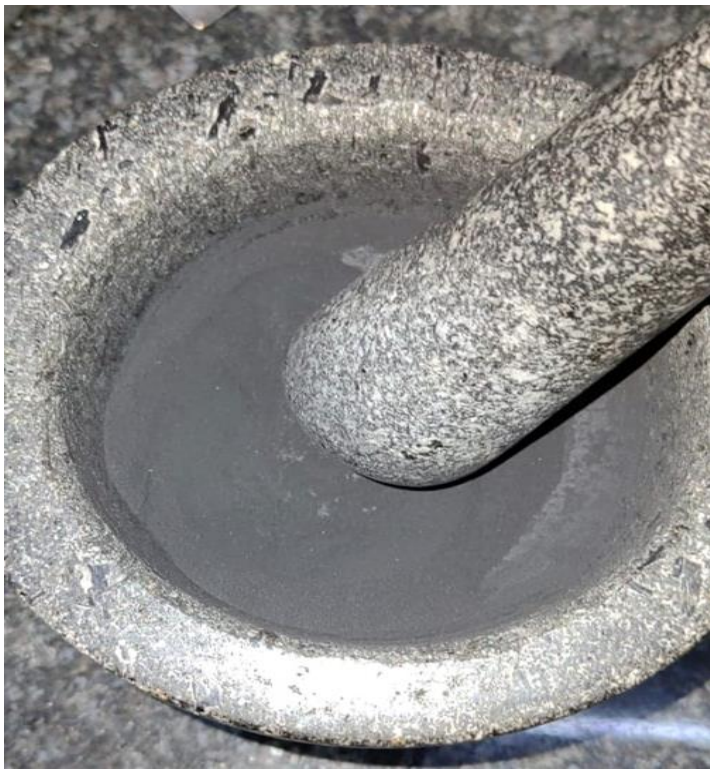
Figure C.4: Method used to mix the coal and binder
