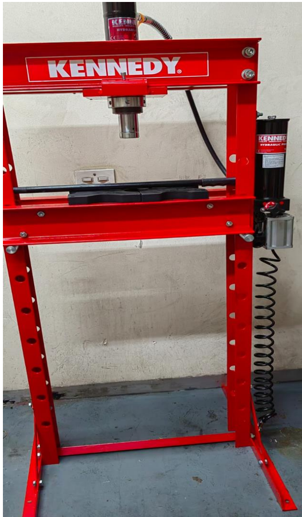
Figure C.5: Hydraulic press used to compact the composites
