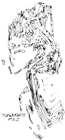
(Plate 25) Conjugate fold in banded ferruginous cherts of the Fig-tree Series west of the Lily Mine. The cherty competent units break angularly while the incompetent shale is moulded between the harder layers. (slightly less than actual size).
