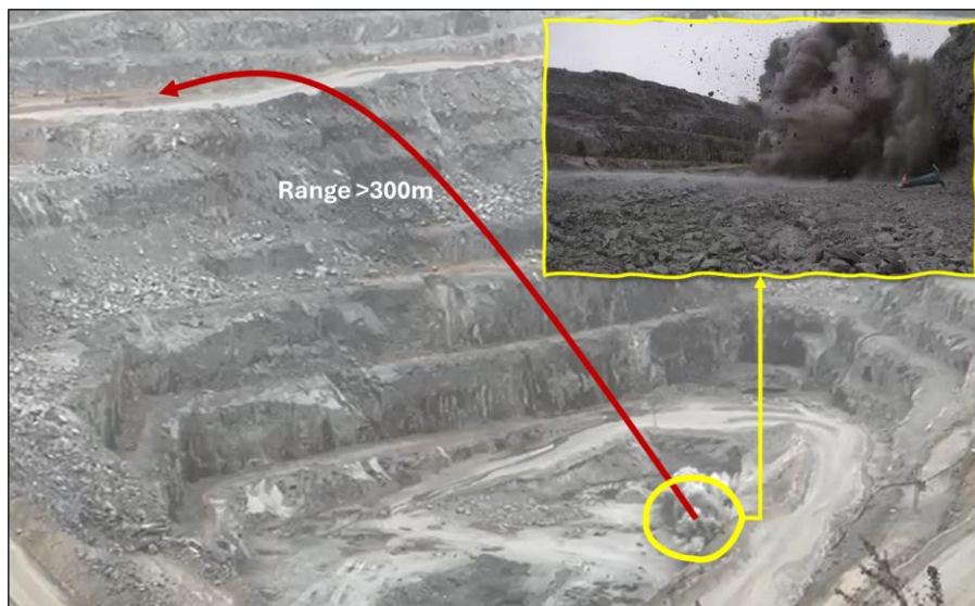
Figure 63: Flyrock from secondary blasting
