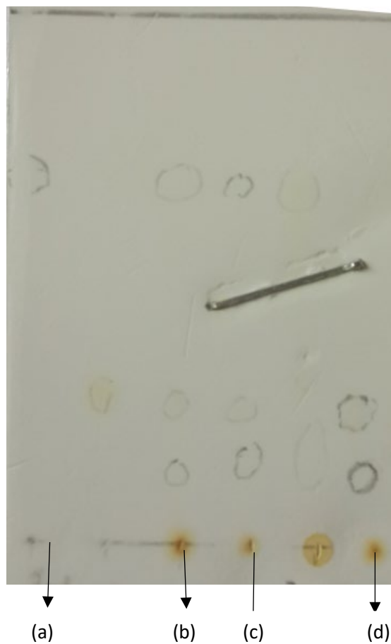
Figure A28. TLC for reductive amination of 54b using diamine donor (40% EtOAc/Hexane). (a) Standard starting material 54d . (b) Reaction involved Prozomix-TA046. (c) Reaction involving Aspergillus fumigatus . (d) Reaction involving prozomix-TA011.
