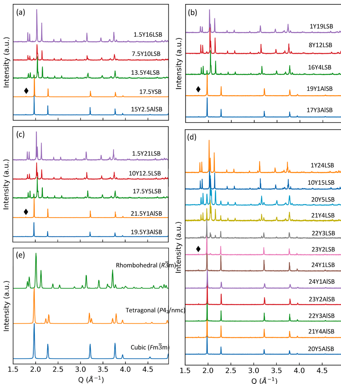
Fig. 3. Room temperature diffractograms of doped bismuthates with (a) 17.5 %, (b) 20 %, (c) 22.5 % and (d) 25 % total dopant content. K_{\beta} reflections are shown with \blacklozenge symbols. (e) Calculated diffractograms of the cubic, tetragonal and rhombohedral phases.
