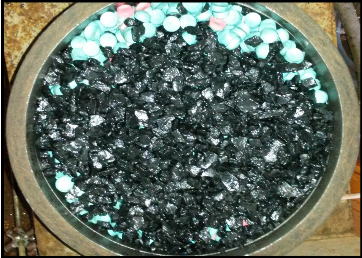
Figure 9: The effect of turbulence in the jig chamber
