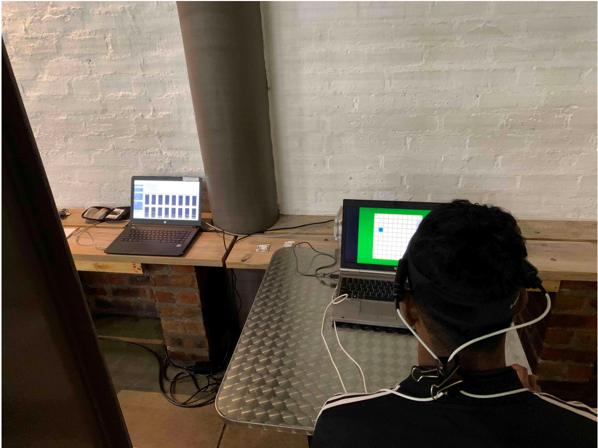
FIGURE 2.5: Participant completing cognitive assessments prior to batting bout. CogState test battery recording user responses to cognitive tests (groton-maze learning task) and second laptop recording raw spectroscopy data from the fNIRS head-band
