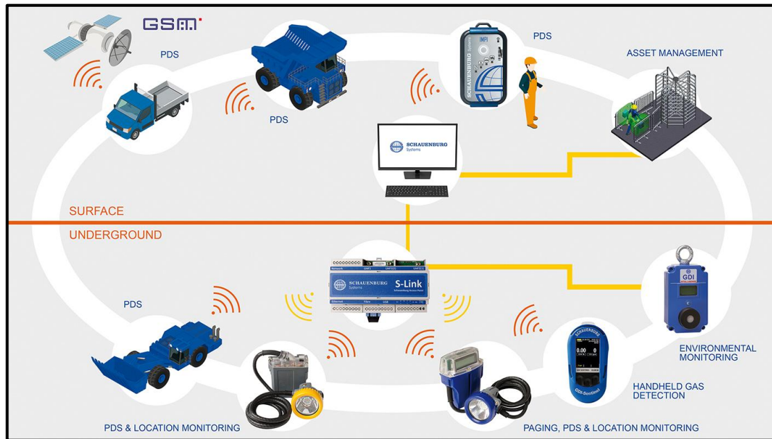
Figure 1-4 Overview of the Schauenburg MIMACS II system (Schauenburg, 2018)
