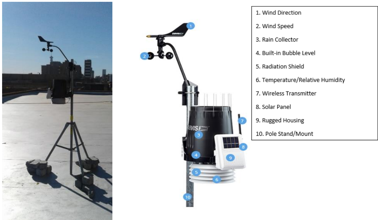
Figure 11. Functions of the Davis Vantage Pro2 weather station (Davis, 2016).
