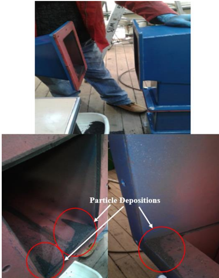
Figure 5 - 1: The particles deposition observed during repeatability testing
