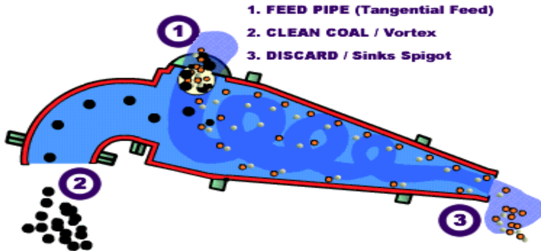
Figure 2 - 2: Basic Working principle of the Dense Medium Cyclones. Image from Parnaby Cyclones, (2015)
