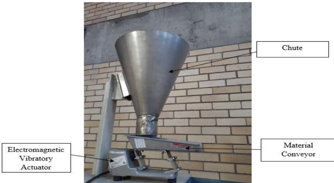
Figure 3 - 12: The Vibratory feeder Assembly
