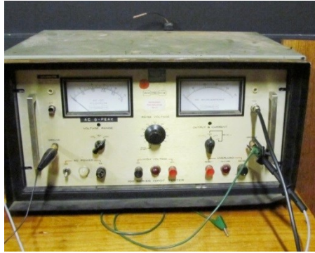
Figure 35: Hipotronics power supply
