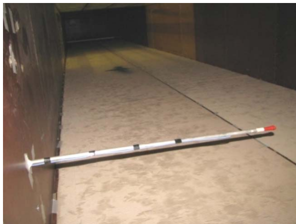
Figure 3.8 - Upwind fetch (‘rough’ boundary-layer)
