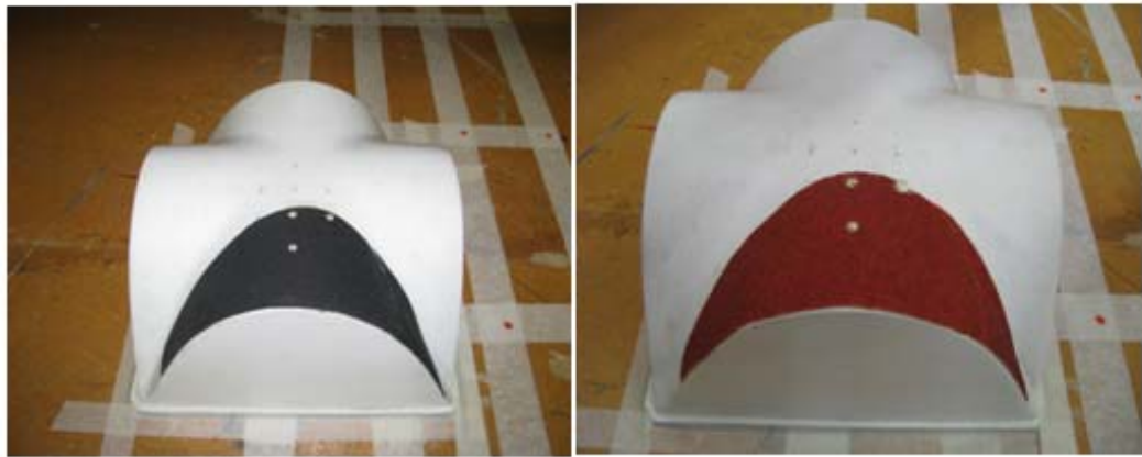
Figure 4.2 - P150(left) and P40(right) grit sandpapers attached to the model
