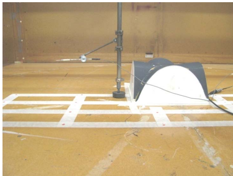
Figure 3.17 - Dynamic pressure measurement at roof height
