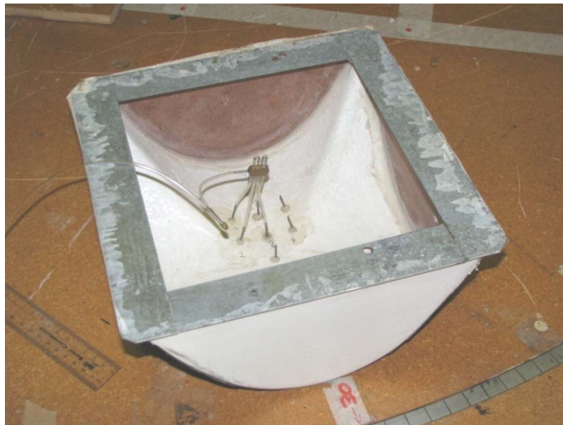
Figure 7.1 - Manifold attached to the flat cross vault
