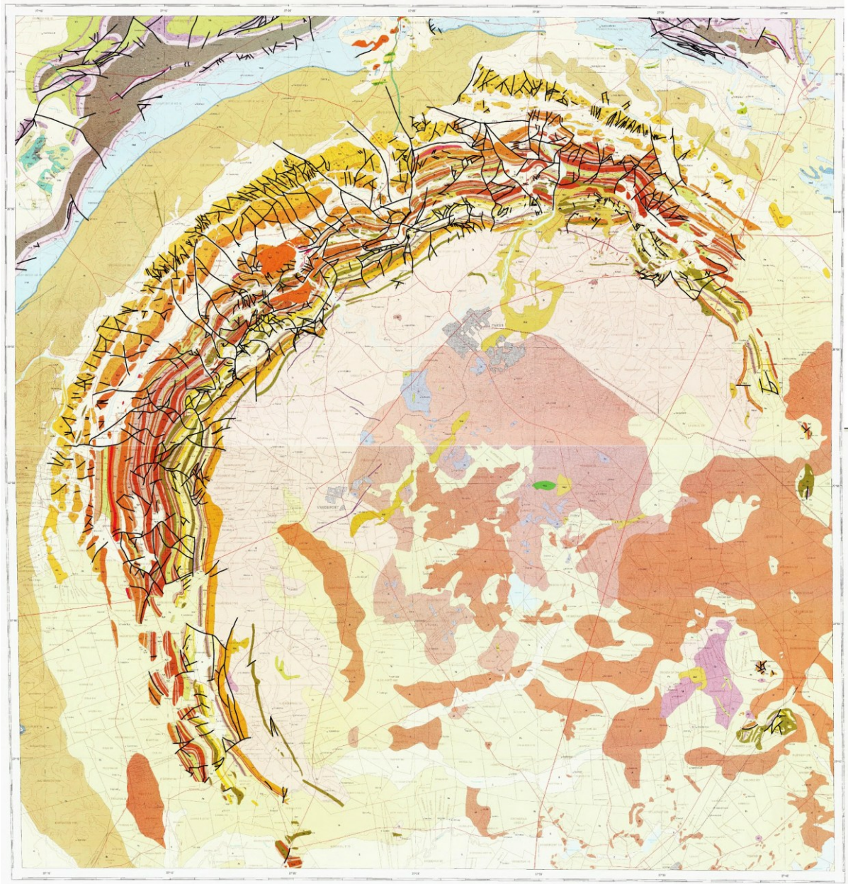
Figure 0.9: Geological Map of the Vredefort Dome by Bisschoff (2000) with digitised fault traces shown in black. Visually, two corners appear in the collar-basement contact at 040° and 270°; however, these do not continue centrifugally. The formation of rollover anticlines associated with pre-impact D3 faults in the northern collar caused a pre-impact bedding anomaly ( see Chapter 1.3.2 ).
