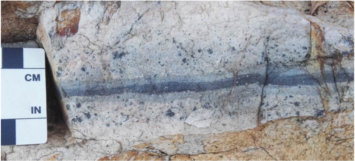
Figure 0.10: Thin pseudotachylyte within cataclasite in Brixton Formation quartzite. Sample RAS-102. Photo location UTM 35J 0537659 E 7028591 S. The dark blue-grey pseudotachylyte shows flow banding and contains visible quartzite clasts. The lower dyke contact is more irregular and diffuse than the upper contact. The lighter grey marginal zones comprise cataclasite. These are flanked by wider zones of discoloured blue-white quartzite that transition into the white quartzite host rock and contain irregular spots of black iron oxide, which are absent from the host quartzite (see Figure 0.13).
