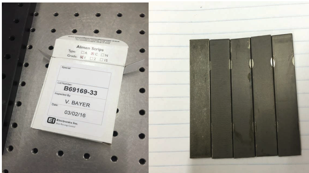
Figure 3-1. Some of the Almen strips that were used to obtain the LSPwC parameter trends
