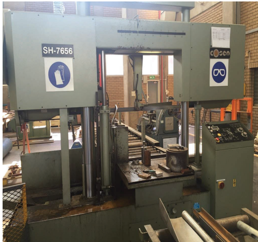
Figure 3-9: The band saw used to machine turbine blade
