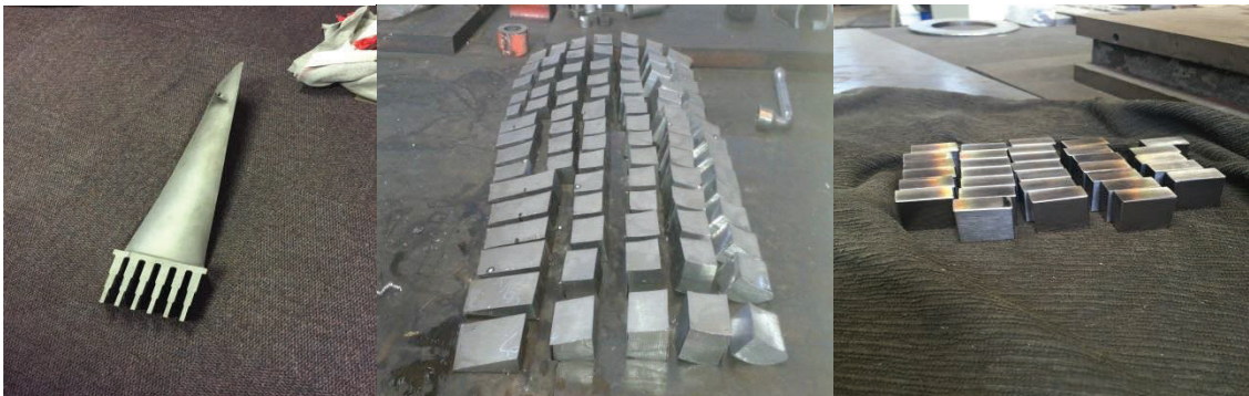
Figure 3-4. Photographs of the blade before and after machining
