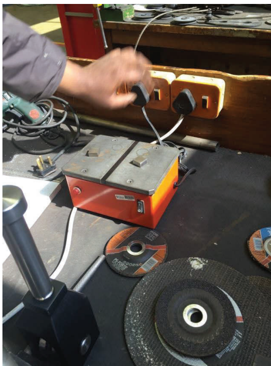
Figure 3-12: Samples on the demagnetising machine
