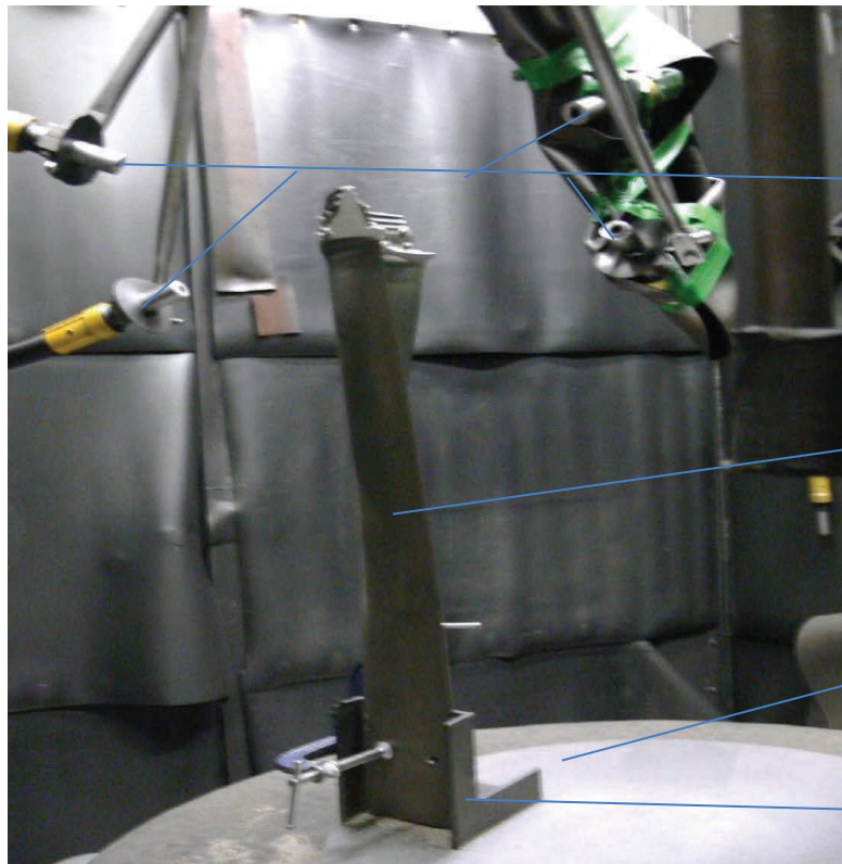
Figure 3-21. Setup extracted from (Newby, 2012) depicting how the sample is placed inside the shot peening chamber.
