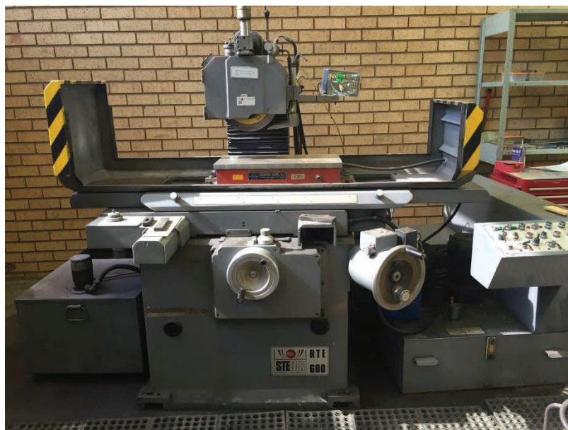
Figure 3-11: Sanding machine used to achieve the final 10mm thickness dimension as well as a smooth surface finish
