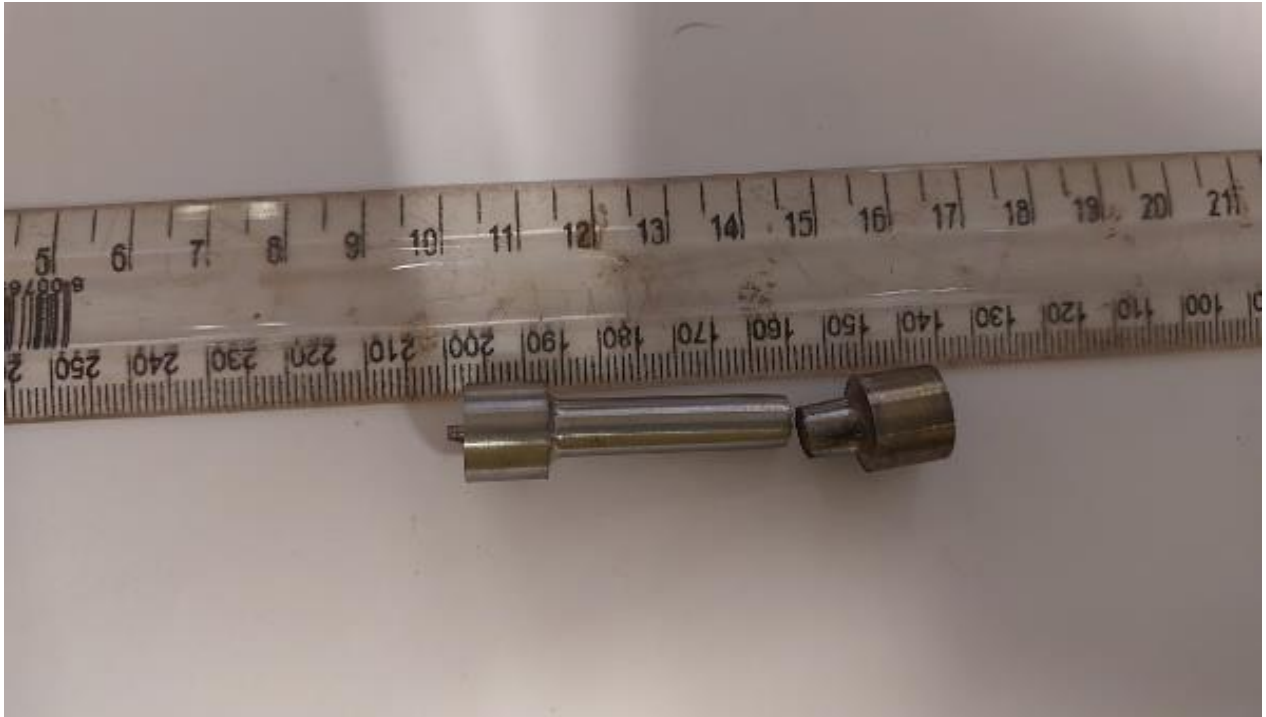
Figure 4-28: Photo showing the sample that was tensile tested on the parent of the head region.
