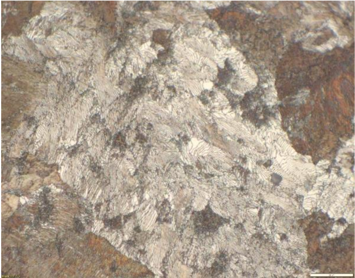
Figure 4-10: Microstructure of a TW R260-60E1 pearlitic rail steel taken on the weld centre. [Etched in 5% nital, 500x magnification].
