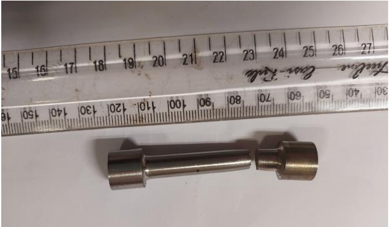
Figure 4-26: Photo showing the sample that was tensile tested on the HAZ of the web region.
