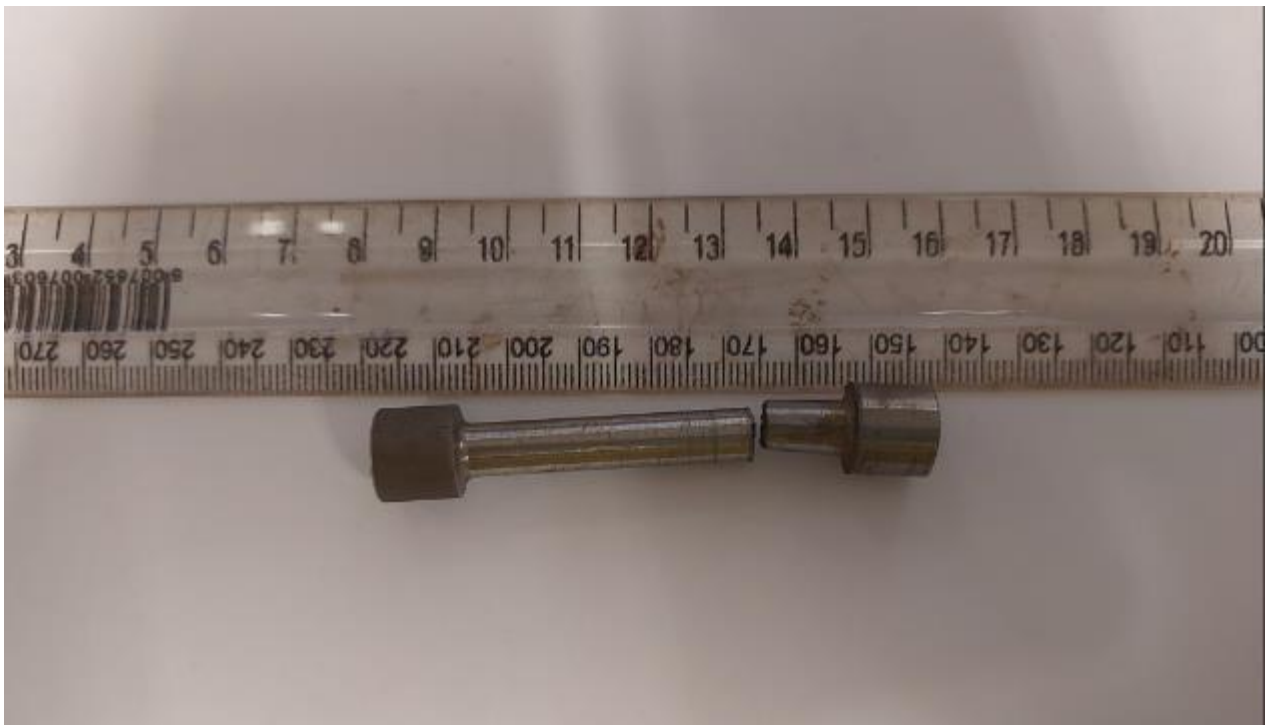
Figure 4-27: Photo showing the sample that was tensile tested on the weld of the web region.
