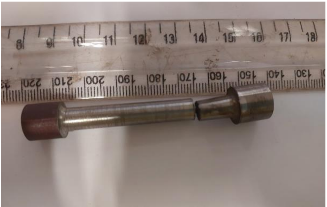
Figure 4-29: Photo showing the sample that was tensile tested on the weld of the head region.
