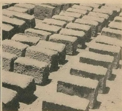
The Kimberley brick, a wood moulded, sun-dried clay brick, measuring 13\frac{1}{2} in. x 9 in. x 5 in.
