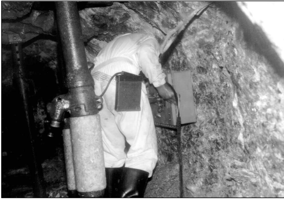
Figure 18: The GPR antenna being dragged along the face to collect data (Grodner, 2001)
