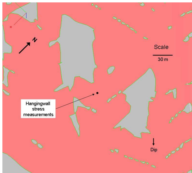
Figure 2-14 Union Site 2: stope sheet showing the location of the vertical hangingwall borehole used to measure the horizontal stress in the hangingwall of a completed stope
