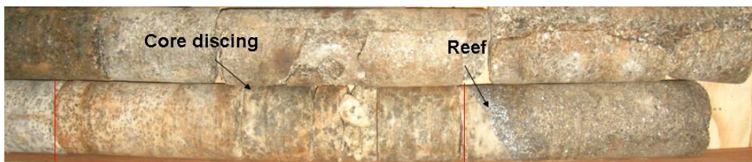
Figure 4-72 Impala site: core-discing observed in the F/W anorthosites
