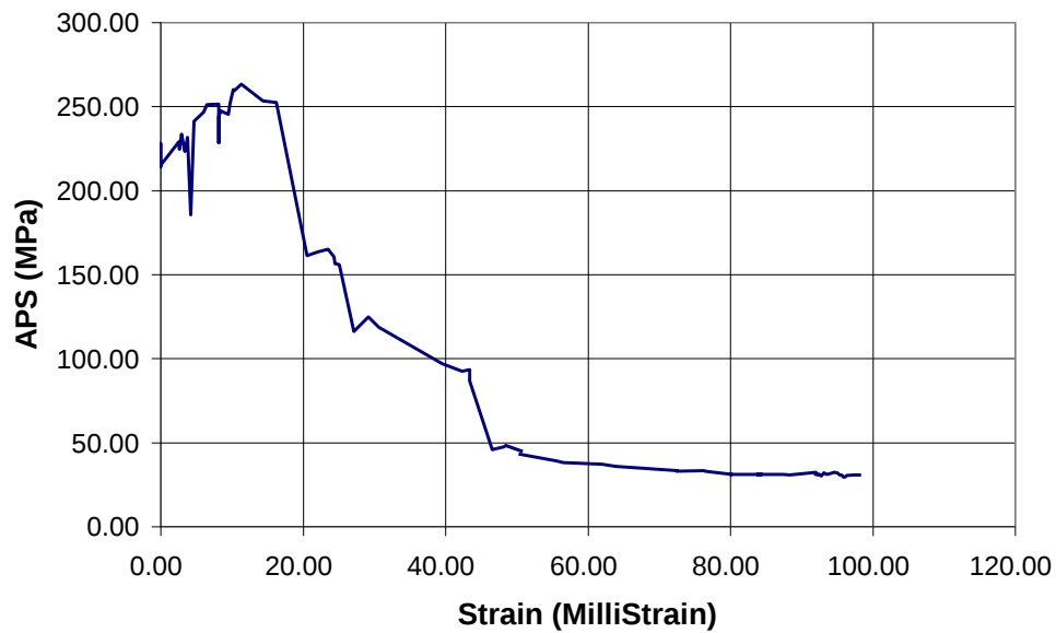
Figure 5-78 Impala site: P3 stress-strain curve using the derived APS values shown in Figure 5-77 and a closure station adjacent to the pillar
