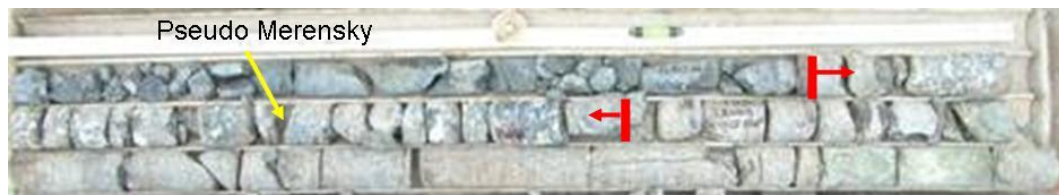
Figure 4-80 Union site: core from the extensometer borehole, showing the fracturing/discontinuities in the Pseudo Merensky
