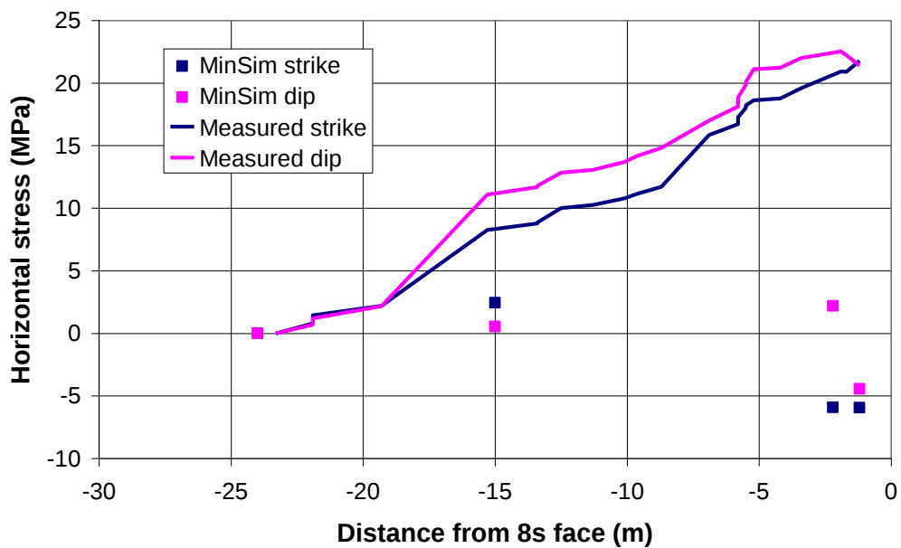
Figure 4-47 Impala site: horizontal stress change 4.2 m above Pillar 2 in Borehole CSIRO1. Negative face positions are behind the cell
