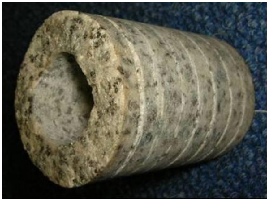
Figure 5-52 Core-discing that occurred about 5.5 m above the proposed P2a position, 2 m ahead of the face
