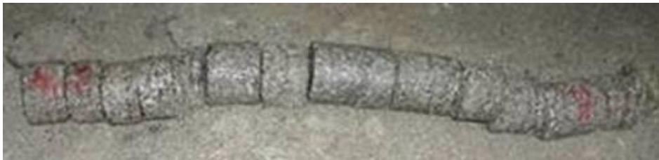
Figure 5-47 Discing of core from the borehole used to install the straincell above Amandelbult P1
