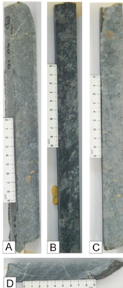
Figure 2.6: Typical lithologies from core AMK-021. A – Feldspathic Pyroxenite (90.25 m depth), B – Serpentinite (222.06 m depth), C – Pyroxenite (232.62 m depth), D – Timeball Hill Quartzite (393.33 m depth).
