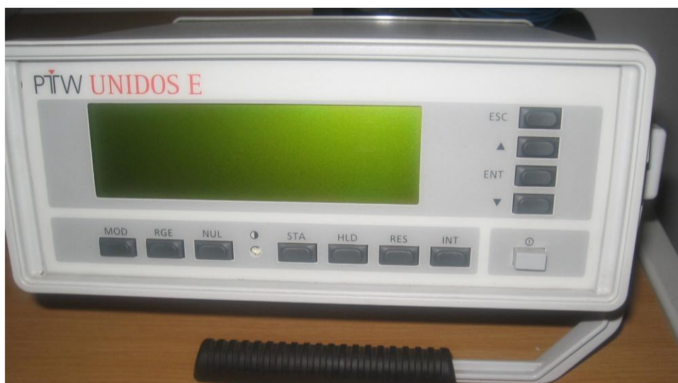
Figure 5.4: The PTW UNIDOS E for biasing the diados and displaying the results of the dose measured
