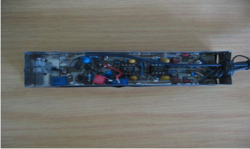
Figure 3.1: Locally designed preamplifier used for alpha spectroscopy
