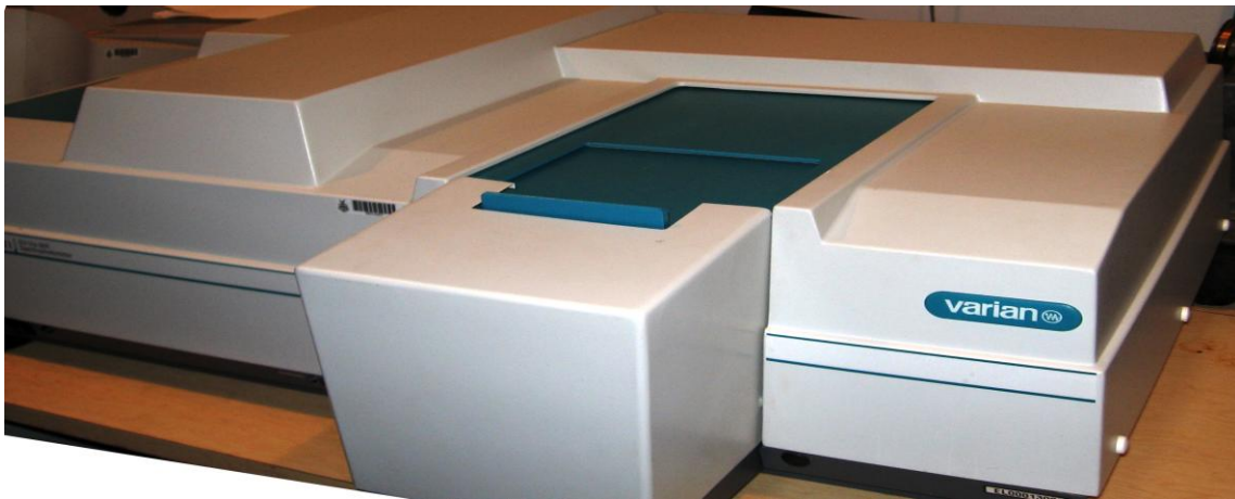
Figure2.7: Ultraviolet scanner model Varian Cary UV-Vis-NIR used for UV absorption
