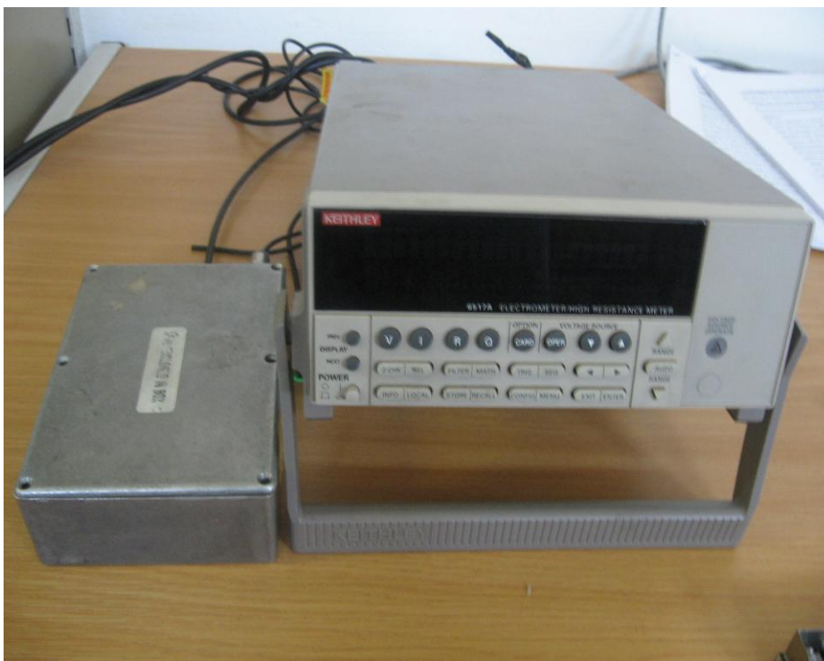
Figure 3.4: Keithley 237 unit and a Faraday cage used for current leakage measurements
