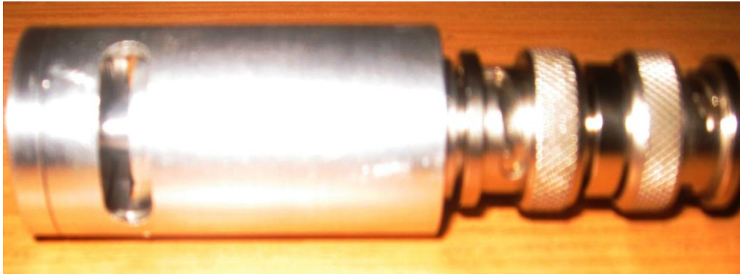
Figure 5.1: The sample holder with BNC connector. The slit opening provides for both positioning and 'edge-on' exposure.
