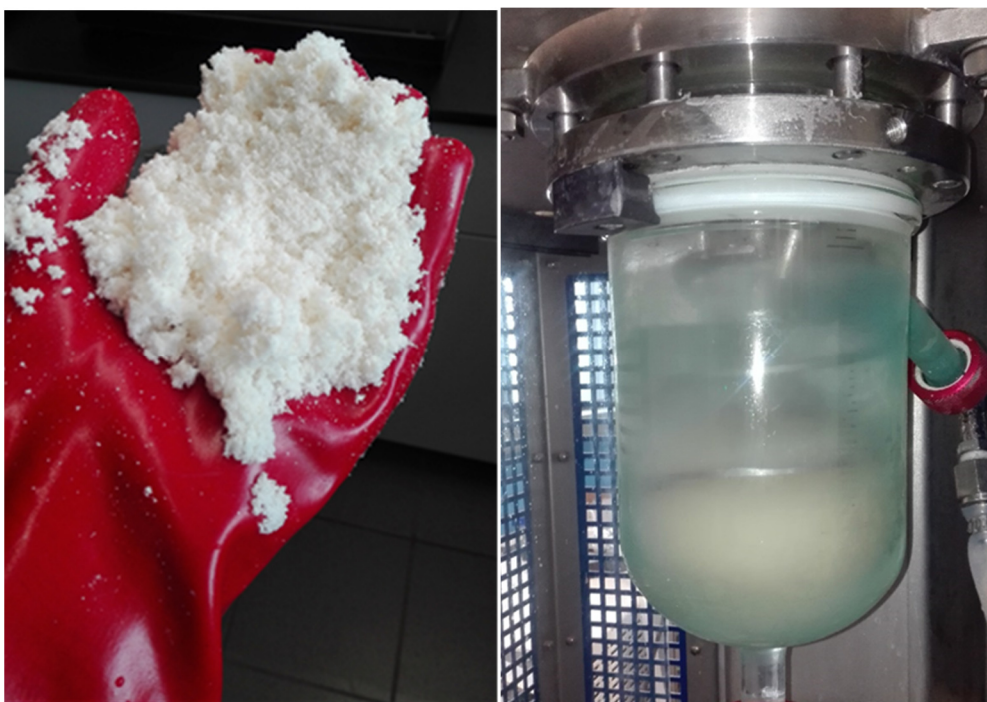
Figure 1-7 Photos of the dry/aqueous reaction (left) and the solvent slurry reaction (right). The dry/aqueous reaction has no free liquid present while for the solvent slurry reaction there is a clear solid liquid separation between the cellulose (bottom) and the solvent (top) when the agitator is stopped.
